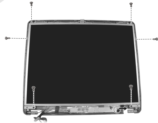
Figure 2-22 Remove the six screws and disconnect the cable
