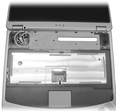
Figure 2-27 Disconnect the four cables
