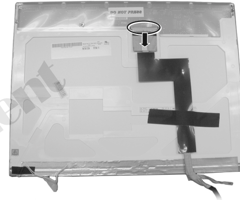
Figure 2-24 Free the LCD panel
