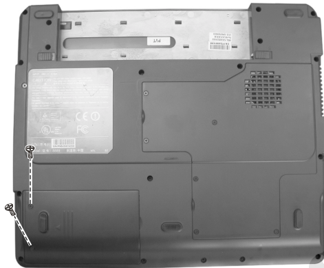
Figure 2-9 Remove the HDD compartment cover
