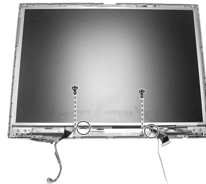
Figure 2-15 Remove the inverter board
